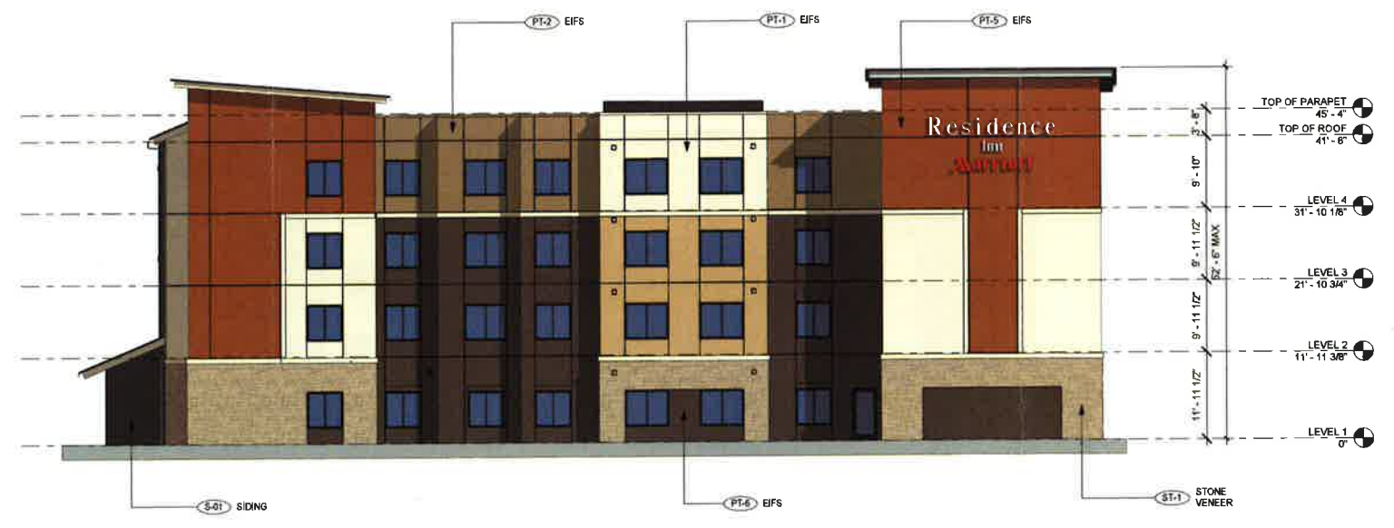
2 EXTERIOR NORTH ELEVATION 3/32" = 1'-0"
