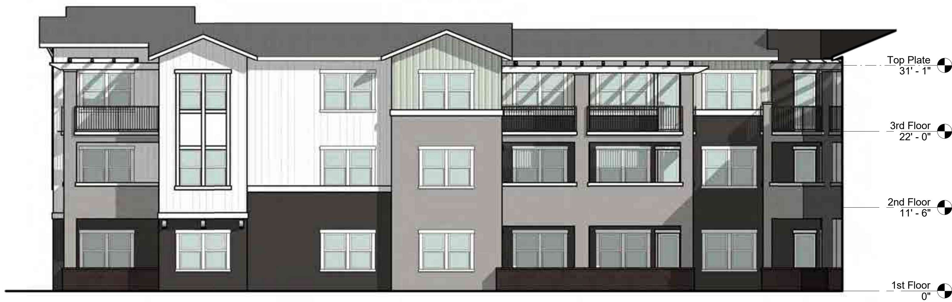
EAST COURTYARD ELEVATION - SOUTH | 2 1/8" = 1'-0"
