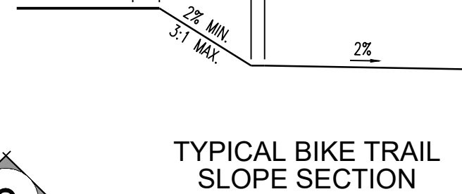
TYPICAL BIKE TRAIL SLOPE SECTION N.T.S.
