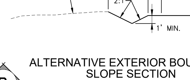
ALTERNATIVE EXTERIOR BOUNDARY SLOPE SECTION N.T.S.
