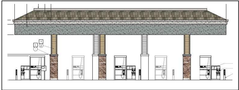
Figure 5: Fuel Canopy Elevation
