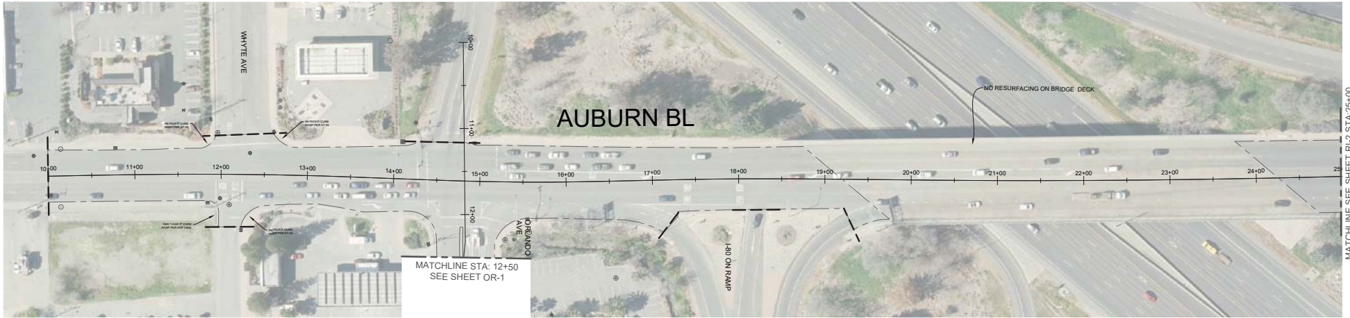
RESURFACING AND DIGOUT LIMITS
