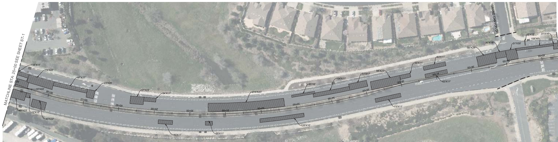
RESURFACING AND DIGOUT LIMITS
