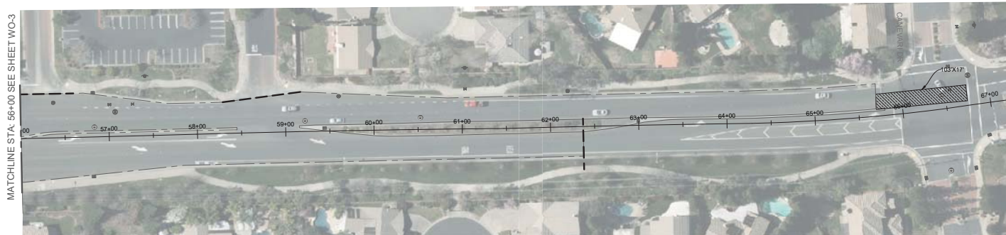
RESURFACING AND DIGOUT LIMITS
