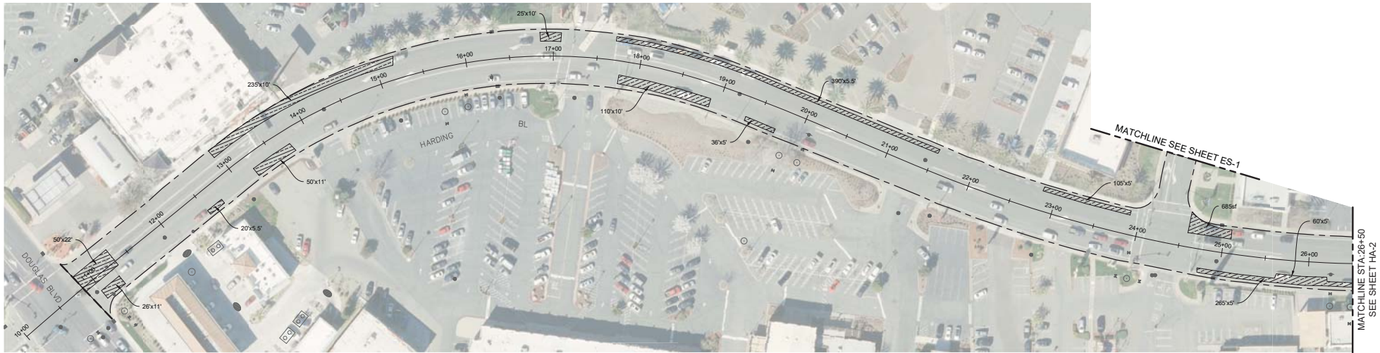
RESURFACING AND DIGOUT LIMITS
