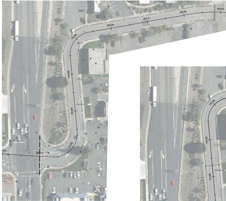
RESURFACING AND DIGOUT LIMITS
