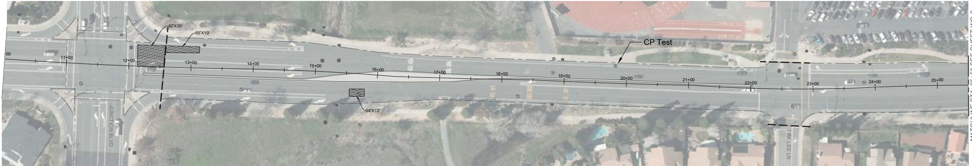
RESURFACING AND DIGOUT LIMITS
