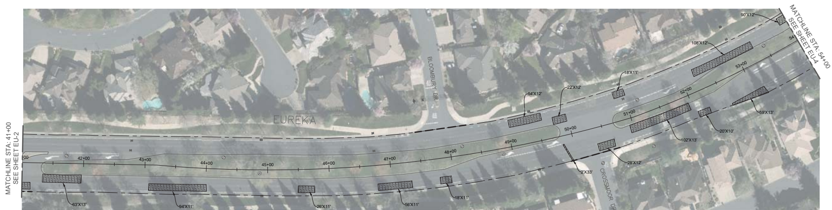
RESURFACING AND DIGOUT LIMITS
