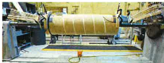
Fully Distributed Regulating Voltage Winding
