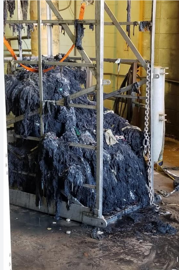
Photo c/o Charleston Water: Fatberg extracted from collection system
