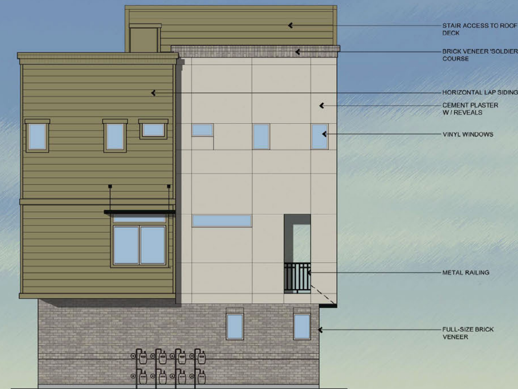
EAST ELEVATION - BUILDING 2 (DRIVE ISLE)
