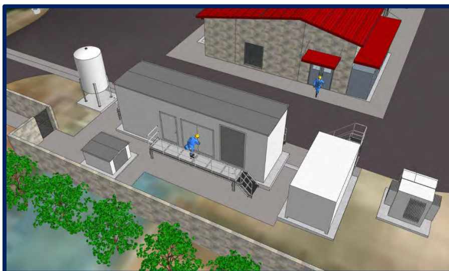
Figure 8: Overview of the current design for a 1500 kW diesel engine generator, load bank, and remote fuel tank located on the east side of the Booster Pump Station.
