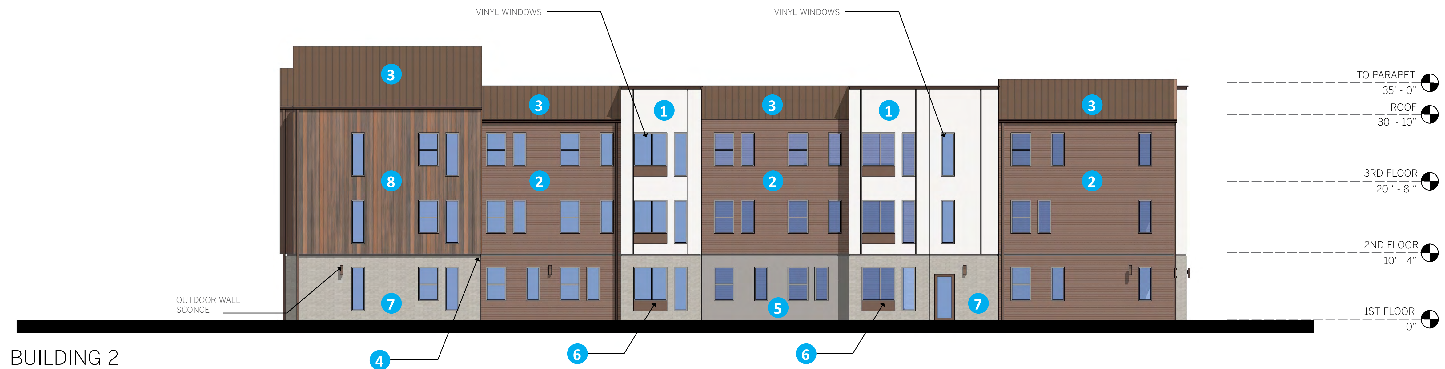
3. METAL PANEL - AEP SPAN FLEX SERIES TERRA-COTTA
