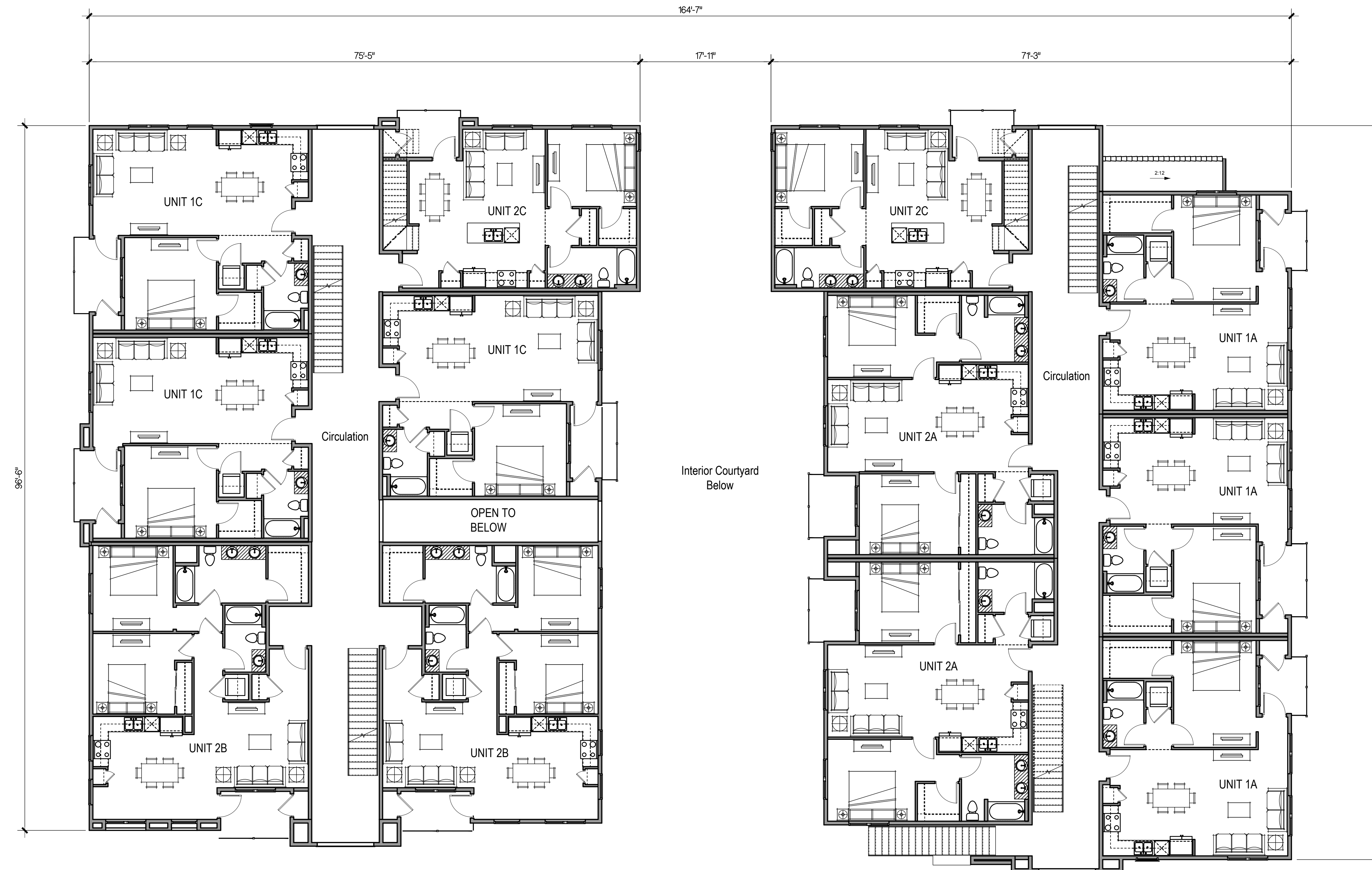
Stack Flat 29-Plex Second Floor Plan Scale: \frac{1}{8} "=1'-0"
