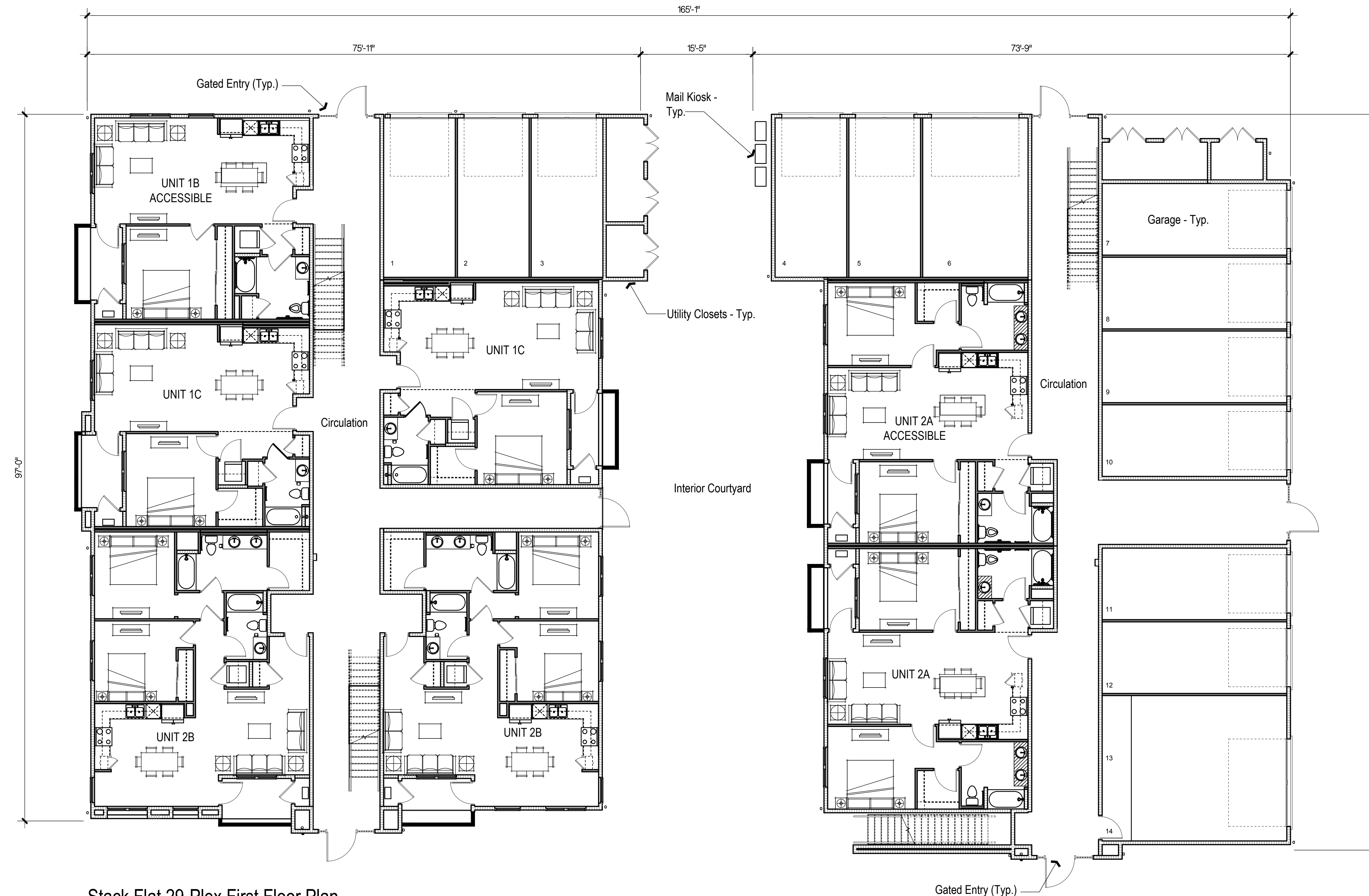
Stack Flat 29-Plex First Floor Plan Scale: 1/8"=1'-0"
