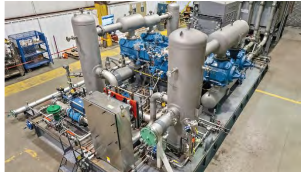
Figure 2: Compass Fuel Gas Compressor
