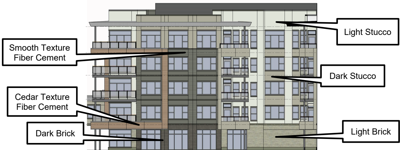
Figure 5. Building RB1.1 North Elevation Materials Detail
