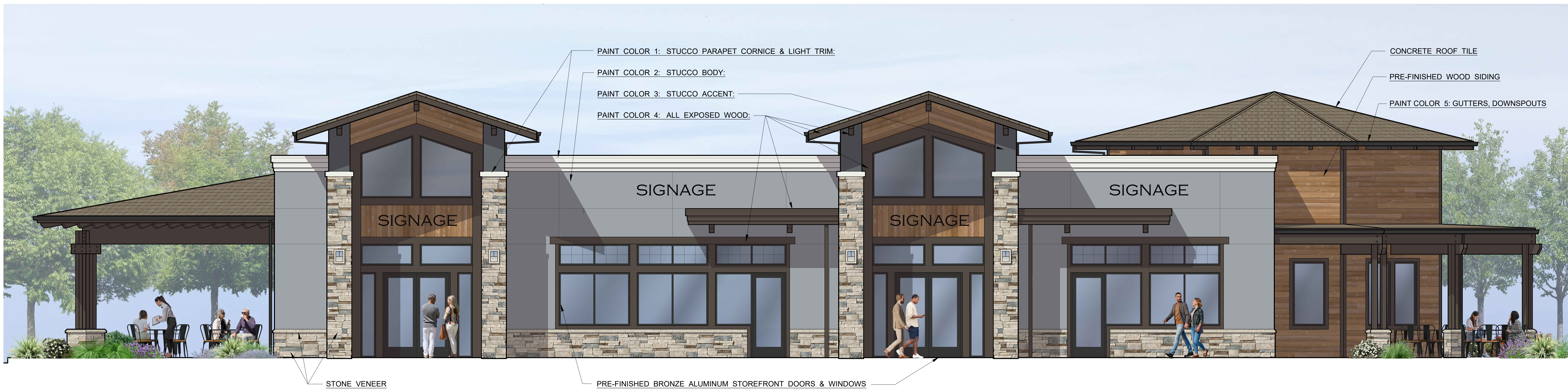
CRAFTSMAN STYLE - EAST ELEVATION FACING PARKING INTERIOR 1/4"=1'-0"
